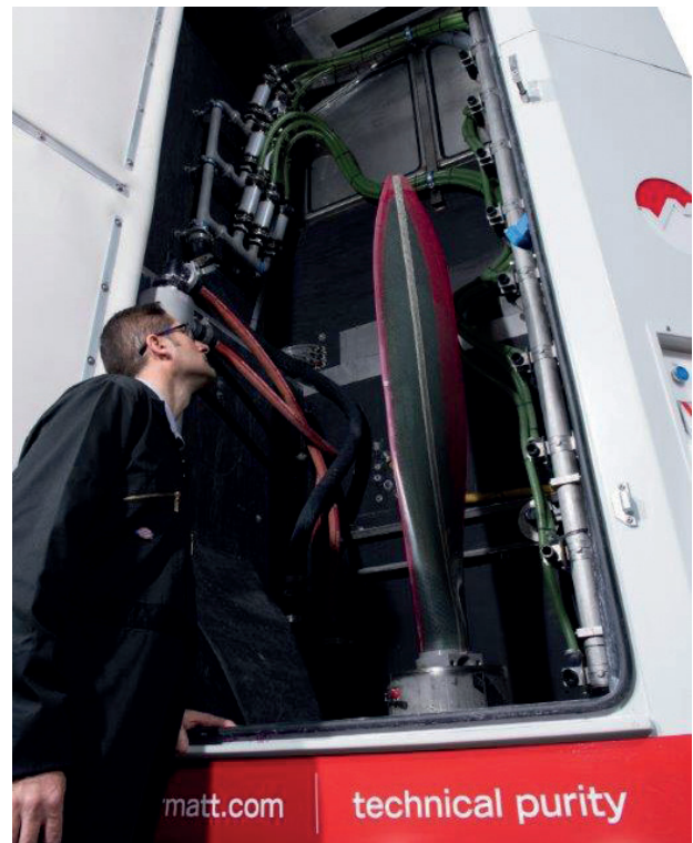
A composite propeller blade about to be processed in a Vapormatt Leopard Cub
