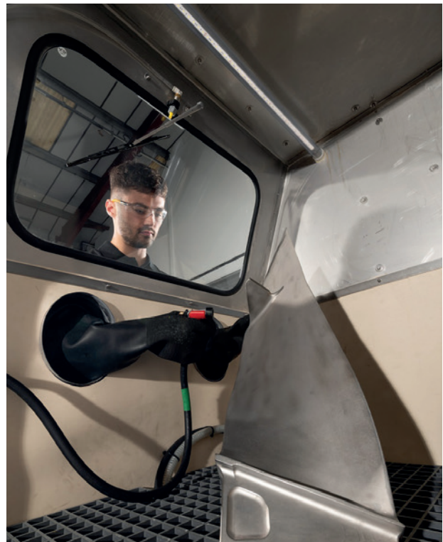
Wet blasting a turbine blade in a Vapormatt Puma
