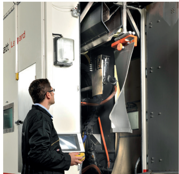
A turbine engine blade being loaded into a Vapormatt Leopard Vertical machine via a holding jig
