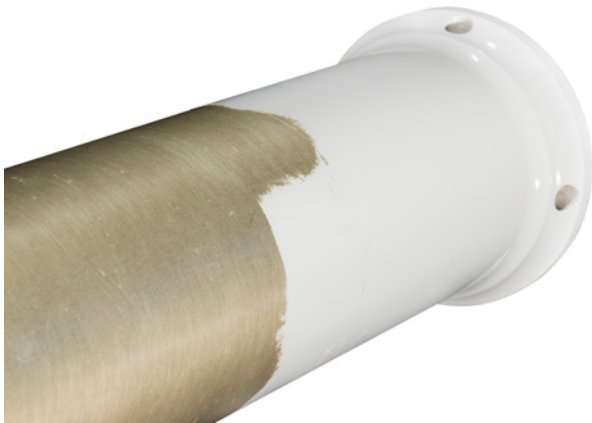
A stainless steel slip coupling that has been paint stripped by wet blasting
