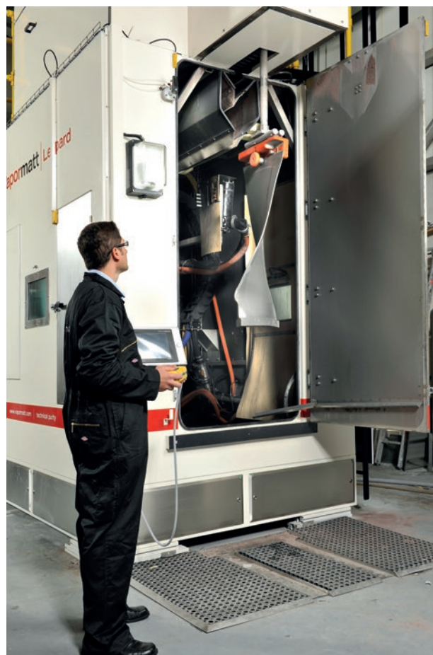
The Vapormatt Leopard can also be used for the peening of turbine blades
