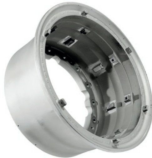
Wet blasting of aircraft wheels is used for crack detection
