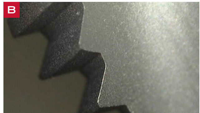
Figure 5: Spiral flute cutting edges before (A) and after (B) processing
