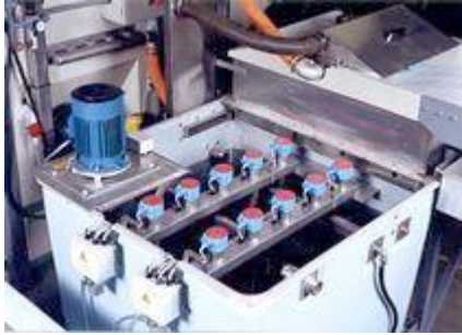
Phosmatt filtration and chemical re-heating tank.
